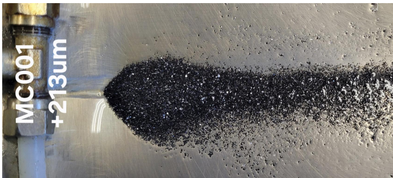
Figure 2: Tantalite concentrate from Mozley table testwork from CV5 drill core composite MC001.
