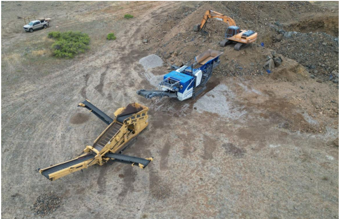
Figure 3 – Aerial view of excavating and crushing at the CSM test pit
