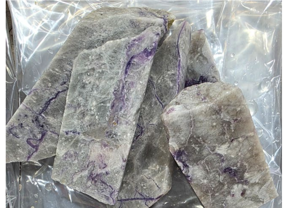
Pollucite core composite (~30% Cs 2 O) from Vega (CV13 Pegmatite). Used as XRT ore sorter training set.
