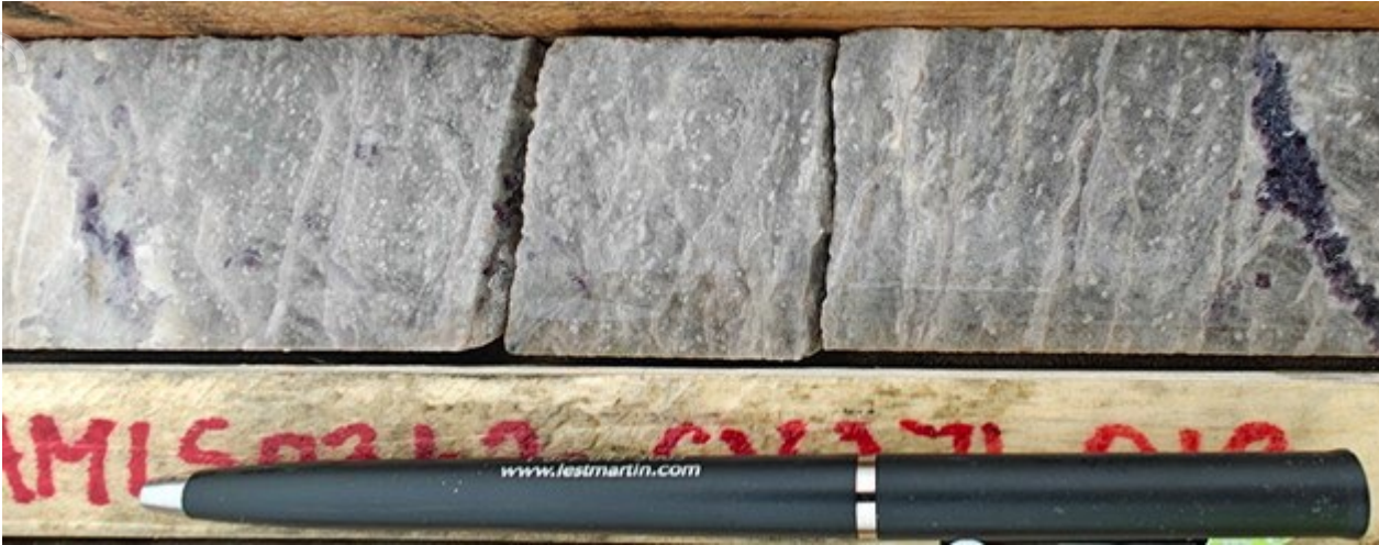
Pollucite mineralization in high-grade caesium drill intersection at ~64.5 m depth in drill hole CV23-271 at the Rigel Zone, CV13 Pegmatite. Interval grades 22.69% Cs 2 O over 1.0 m (64.0 m to 65.0 m) 1
