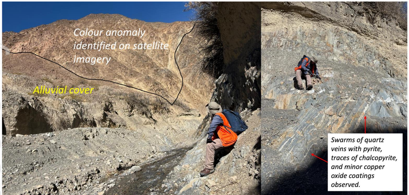
Figure 4: Colour anomaly identified on satellite imagery within Devonian sedimentary rocks at the 1124000630-2024 property. Field inspection confirmed swarms of quartz veins with pyrite, traces of chalcopyrite, and minor copper oxide coatings.
