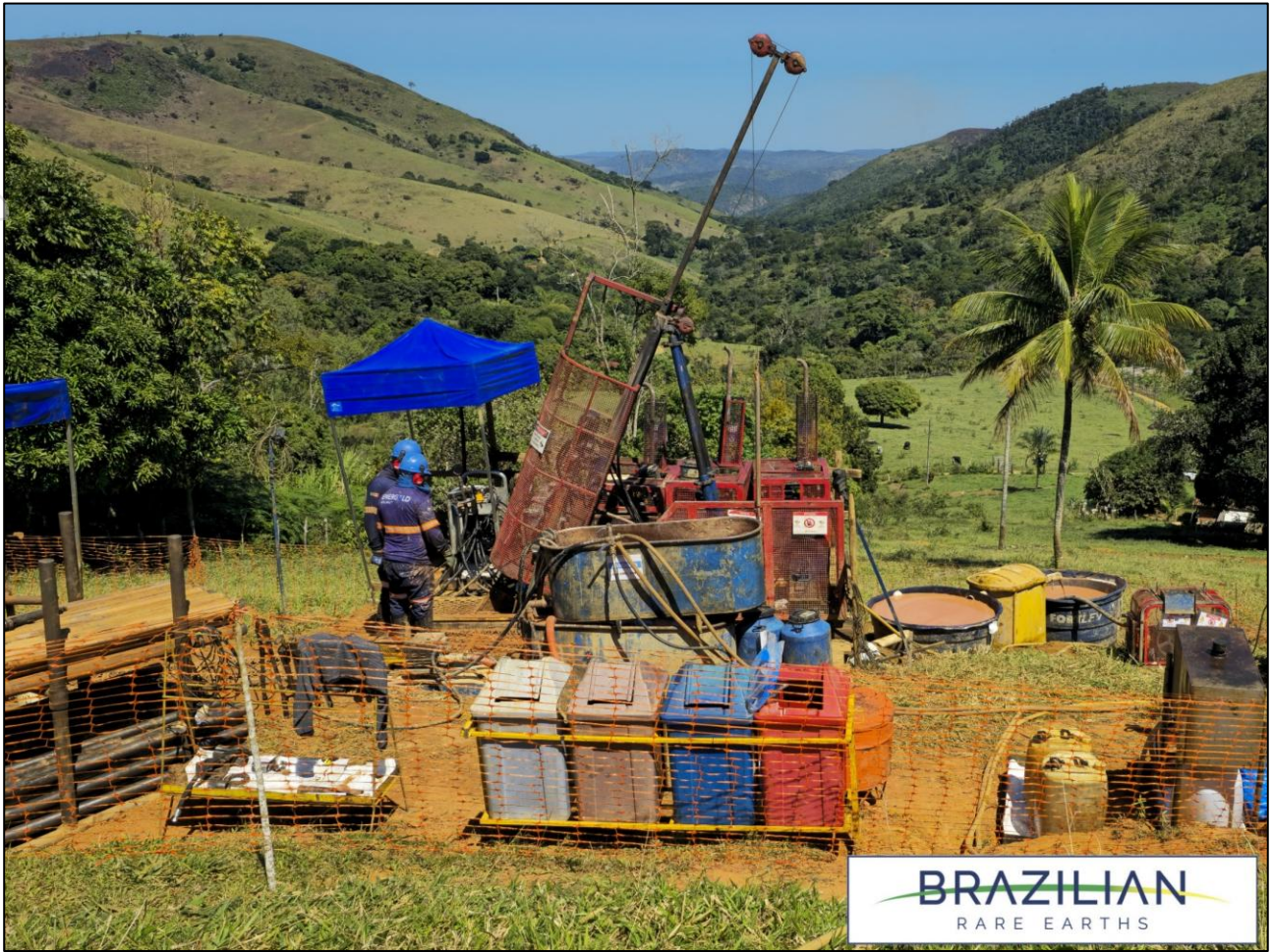
Figure 7: Diamond core drilling at Sulista East
