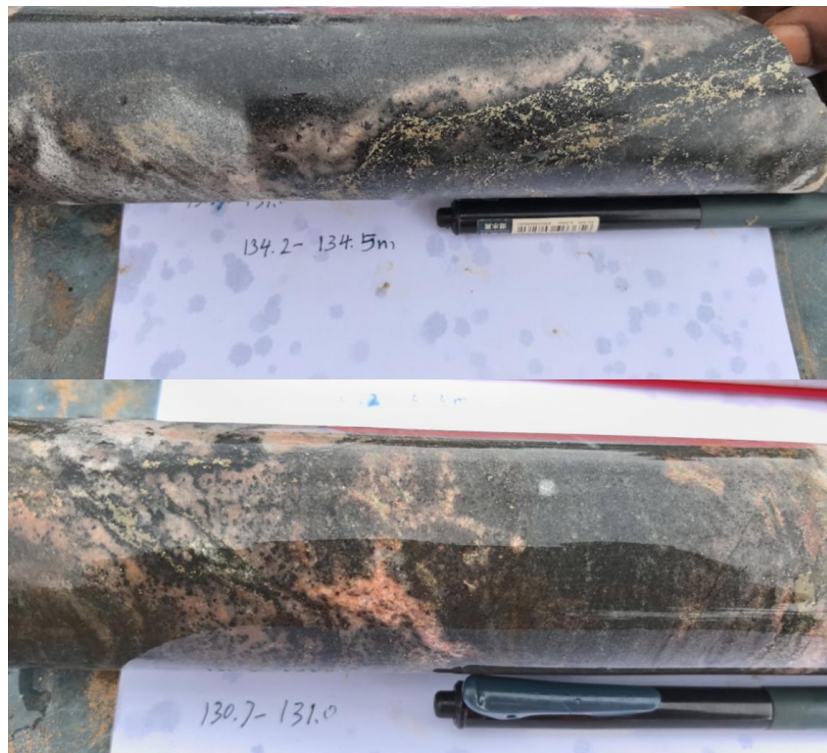
Figure 6. Strong Py observed in the second alteration zone of hole FADD25-001 5
