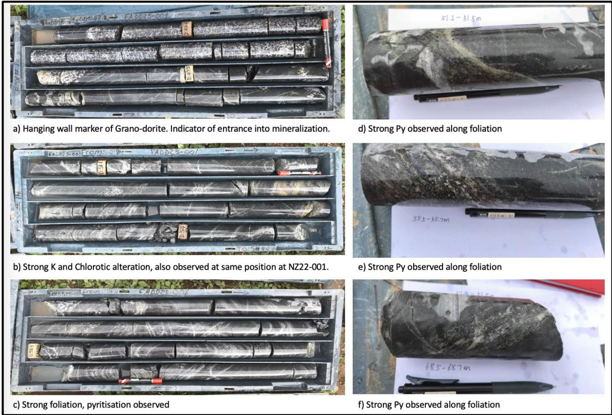
Figure 5. FADD25-001 Intersection from 49.4 – 72.8 m displays similar mineralisation and lithology as up-dip gold discovery intercept in NZ22-001 4
