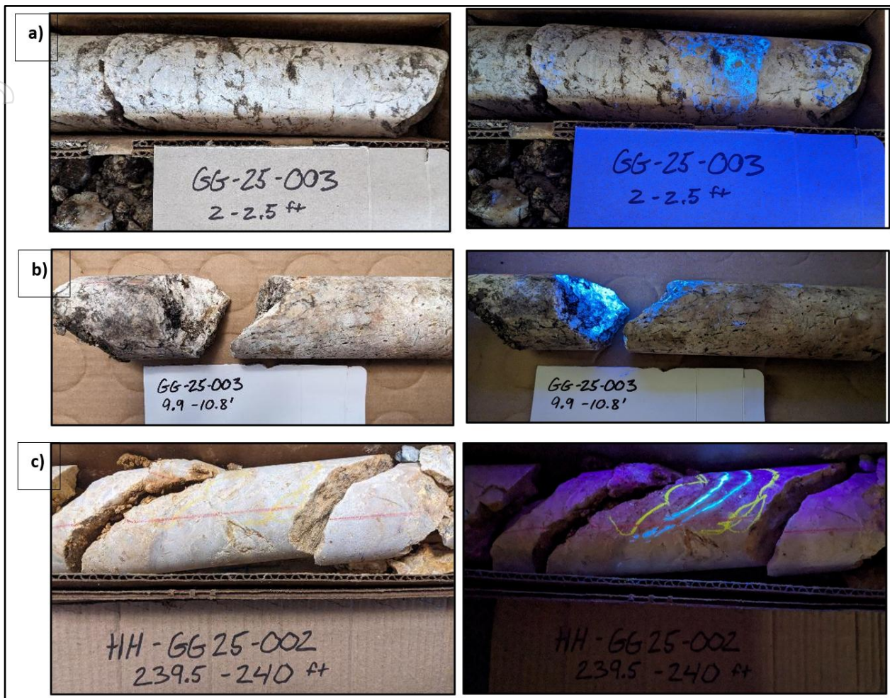
Figure 1: Sections of drill core from Drillholes HHGG25-002 & - HHGG25-003 at the Golden Gate Target of the Horse Heaven Project, with drill core on the left and the same drill core exposed under shortwave UV light on the right indicating the presence of scheelite (tungsten mineralisation \text{CaWO}_3 ). See Figure 3 for the location of the drillholes.
