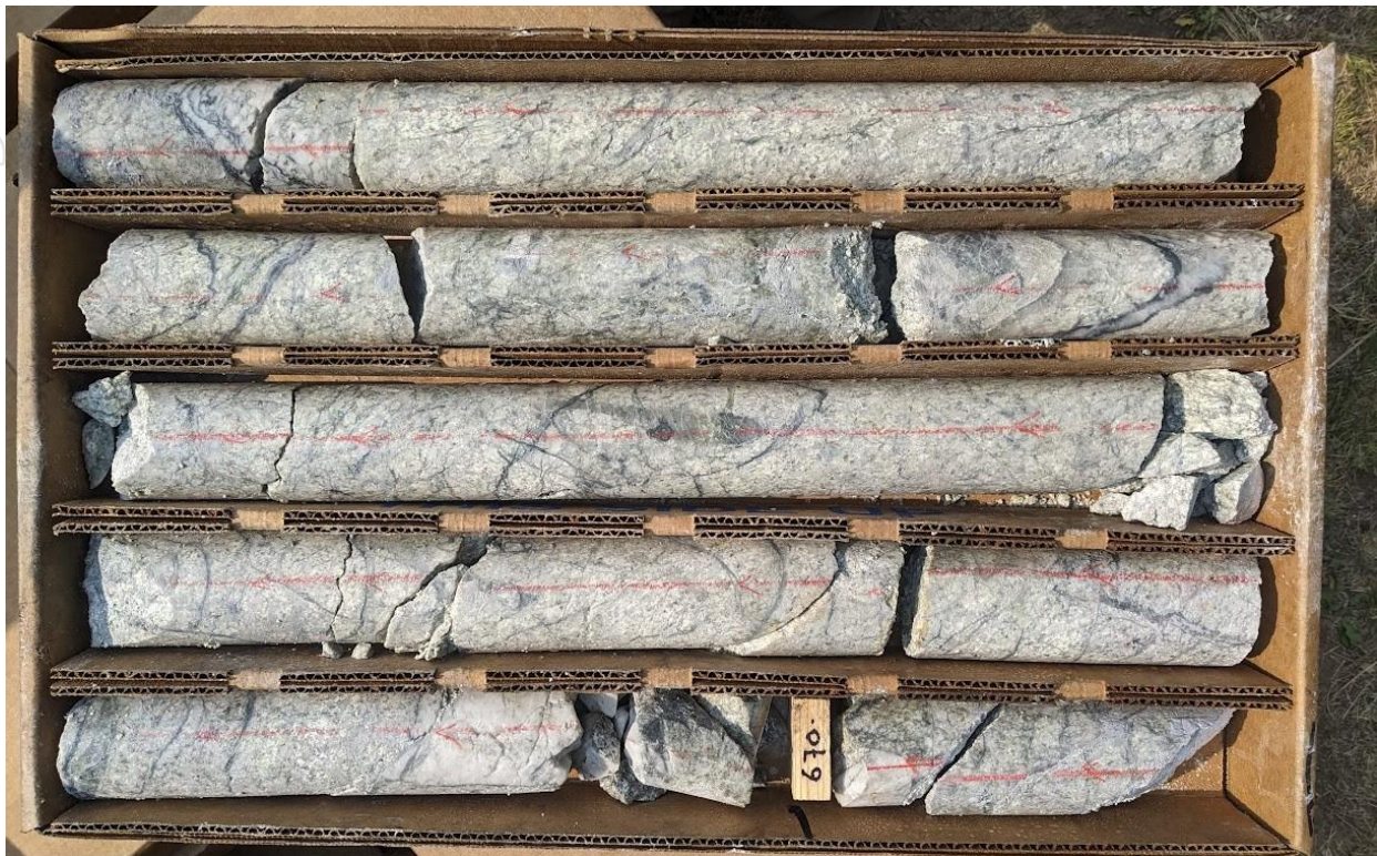
Figure 4: HHGG25-003 drill core at the Golden Gate Target displaying quartz sericite-chlorite altered monzonite with fine grain disseminated sulphides and chalcedonic quartz-sulphide veins and stockworks. Field of view is 60cm (left) and from a depth of 204m to 206.7m (669.2-678.4 ft) in HHGG25-003. This photo of core is included in this announcement to show the high degree of veining and alteration. It does not allude to any form of mineralisation.
