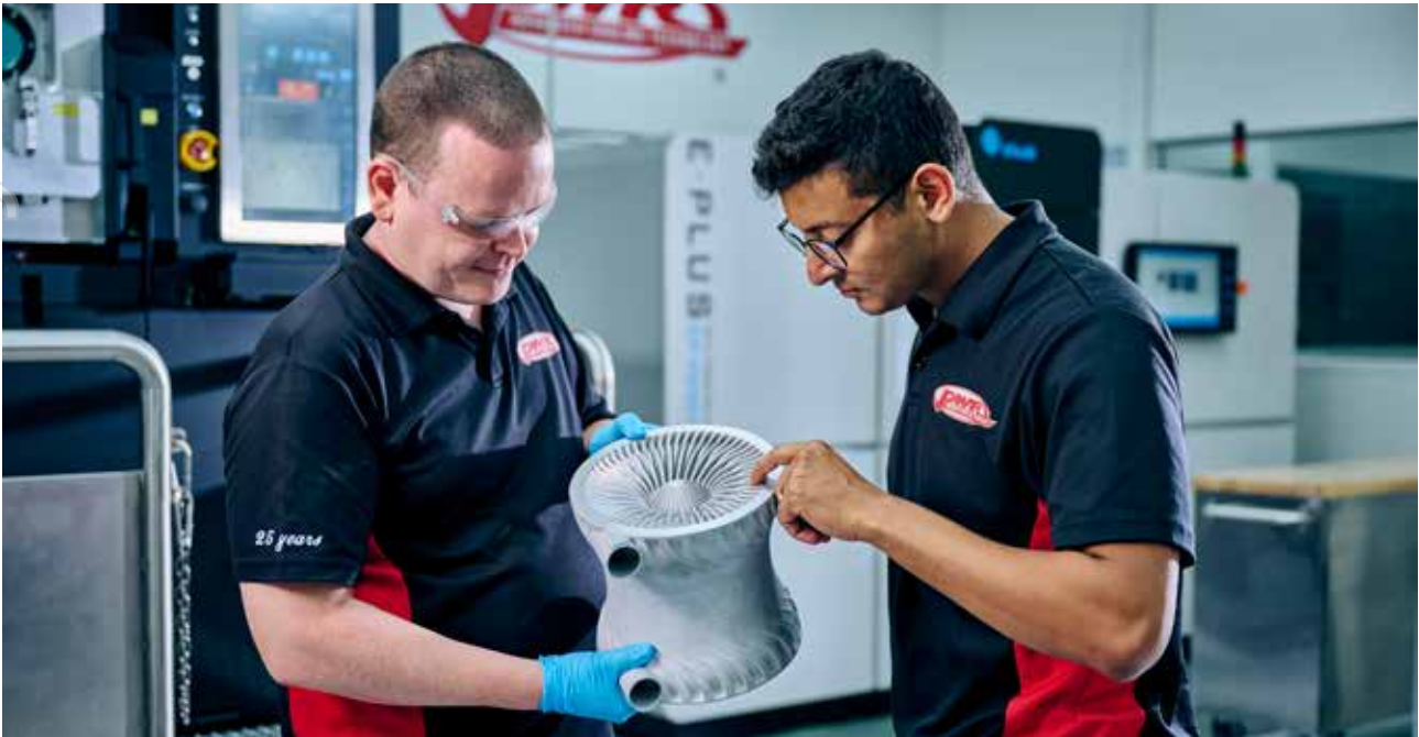
Tobias Maconachie, Additive Manufacturing & R&D Project Lead, and David Yassa, Project Engineer, inspecting an additive manufactured prototype heat exchanger
