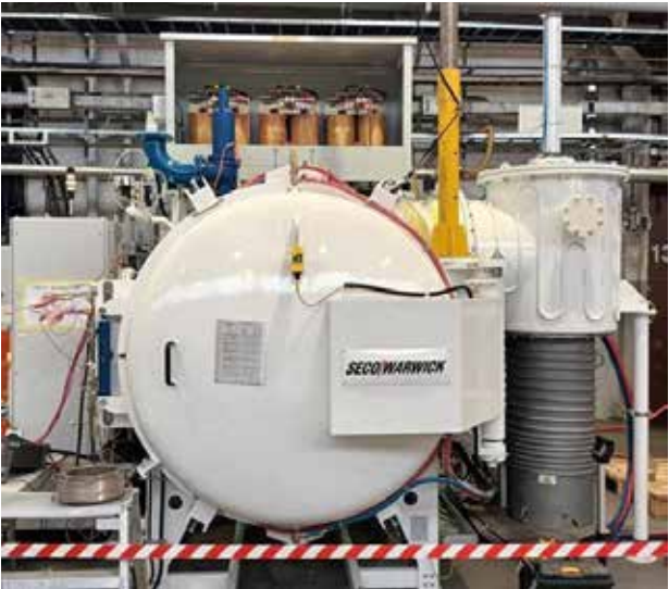
Vacuum braze furnace during factory acceptance testing to 1,200 °C and 5x10 -5 mbar
