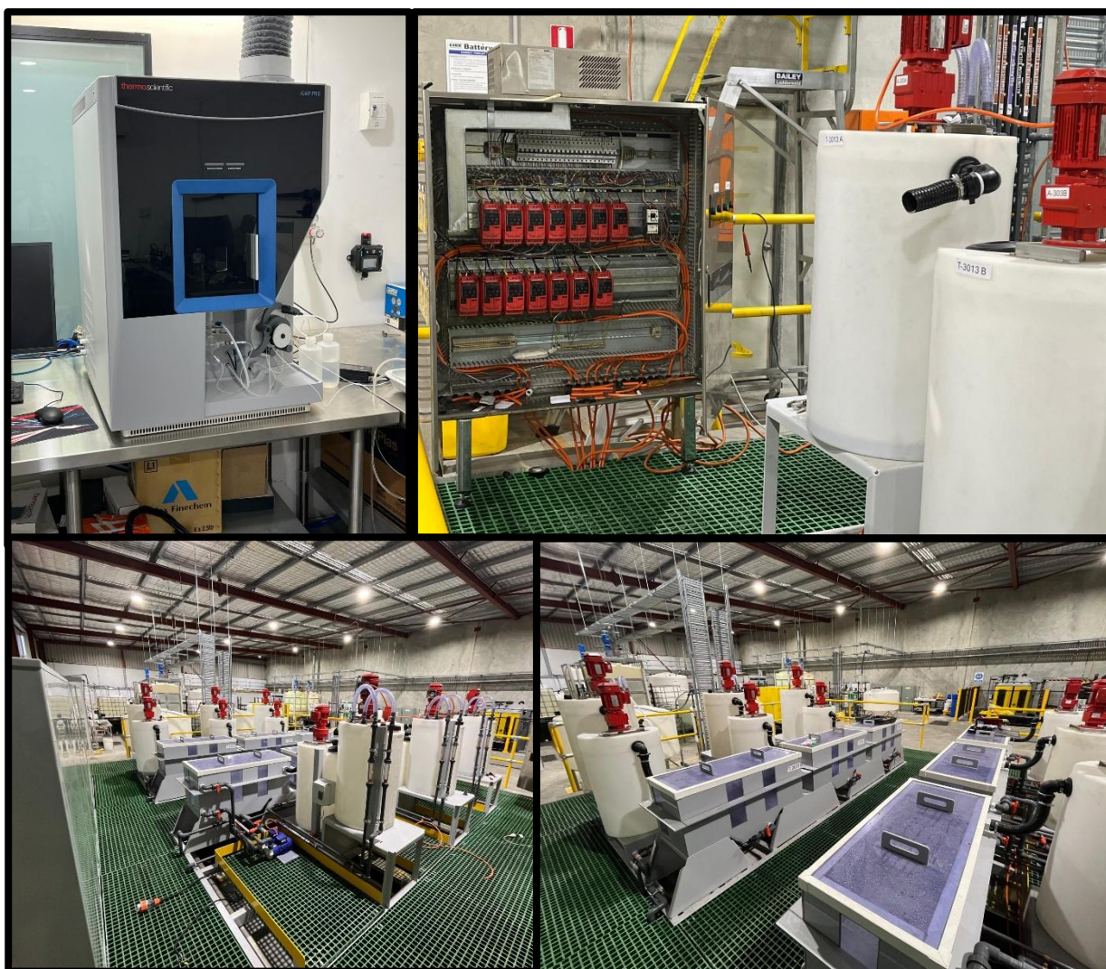
Figure 2. Details of the ICP-MS in the high-purity laboratory, the electrical circuits and the SX circuit)
