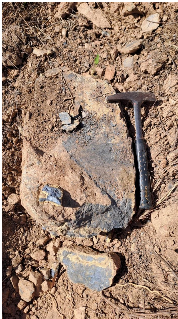
Figure 1; Pacgold rock chip sample SG250704 , Massive Stibnite located near the historical open pit mine at the St George Au-Sb project, Assays returned 49.4% Sb and 0.05g/t Au .
