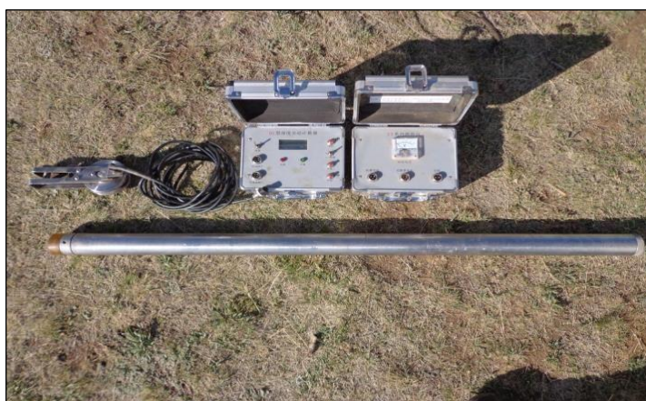
Figure 4-5. GSK 250 K instrument performing well gyroscopic measurement
