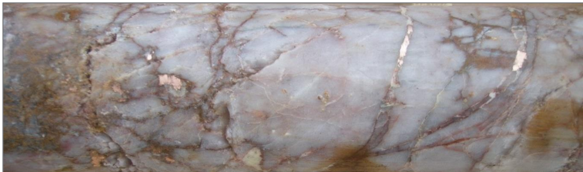
Figure 3-6. Orange copper intersected at 22.3 meters in borehole MUDH-1203.
