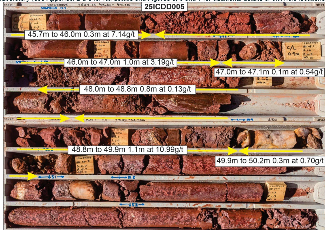
Figure 3 - Drill core from hole 25ICDD005 ( \sim 60 to 083^\circ ), trays 13 and 14 showing sheared and veined gabbro between 45.7m to 50.2m which were assayed and returned a significant intercept of 4.5m at 3.94g/t Au (intervals of core loss are included at 0.0g/t). Photo shows HQ3 (61.1mm diameter) whole-core prior to cutting and sampling. Hole depths & core loss (C/L) are marked on core blocks. Au grades are 50g fire assay as reported by NAGROM laboratory (see Appendix 2 & 3 for full details and Figures 5, 6 and 7 for additional details of drill hole locations).
