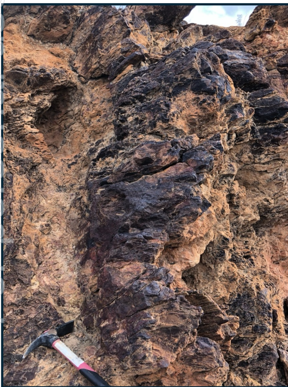
Figure 4 - Copper Zinc mineralised gossan outcropping at Sneaky Squirrel - outcropping mapped along 302m additional sample assays pending
