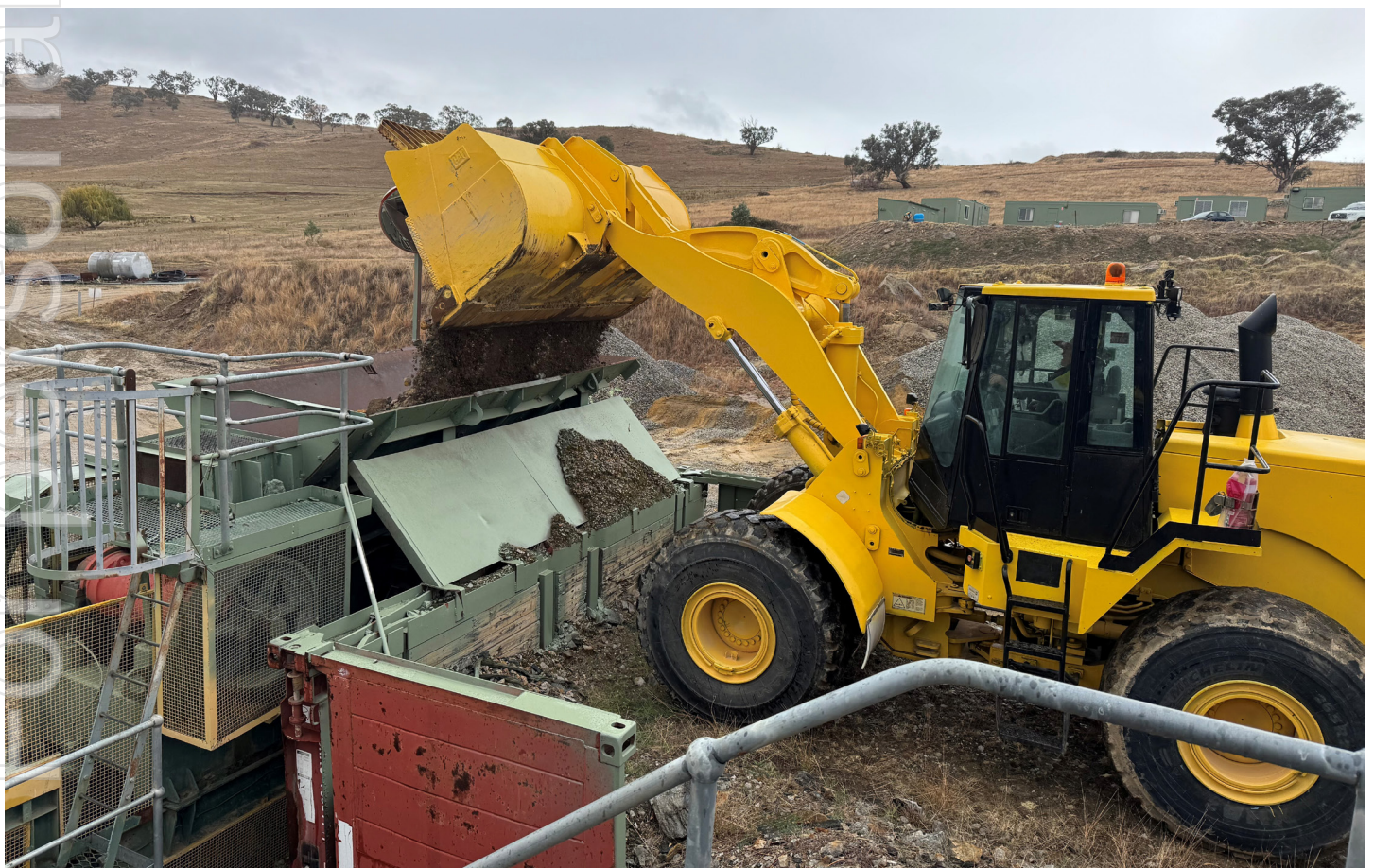
Figure 1: Loader stacking high grade tailings on the Challenger ROM pad ready for feeding to the Gold Plant
