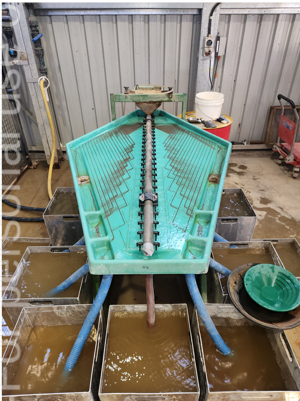
Figure 2: Gemini table refining gold in sulphides concentrates.
