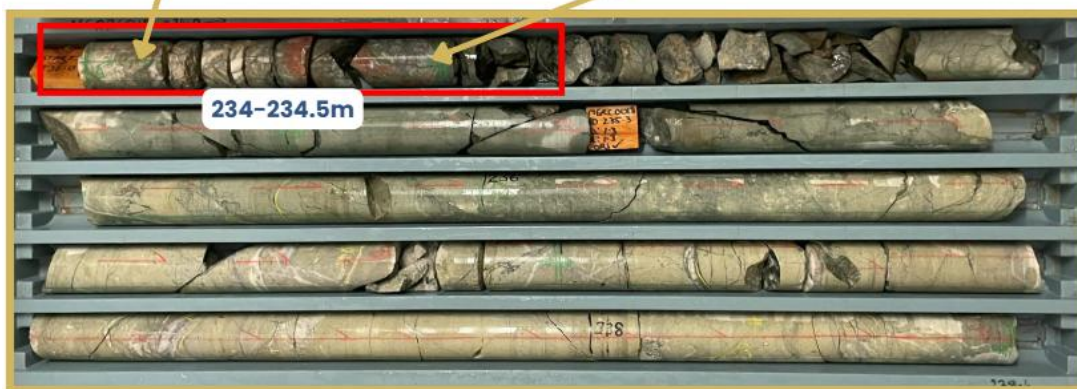
Figure 3: Diamond Tail of MGRC0018 from 234m. Mineralised BIF unit intercepted from 234 to 234.5m, with footwall alteration from 234.5 to 239m. See Appendix B - Table 3 for detailed descriptions and visual estimates. Assays Pending (estimated 4-6 weeks). Cautionary Statement: Visual estimates of mineral abundance should never be considered a proxy or substitute for laboratory analyses where concentrations or grades are the factor of principal economic interest. Visual estimates also potentially provide no information regarding impurities or deleterious physical properties relevant to valuations.
