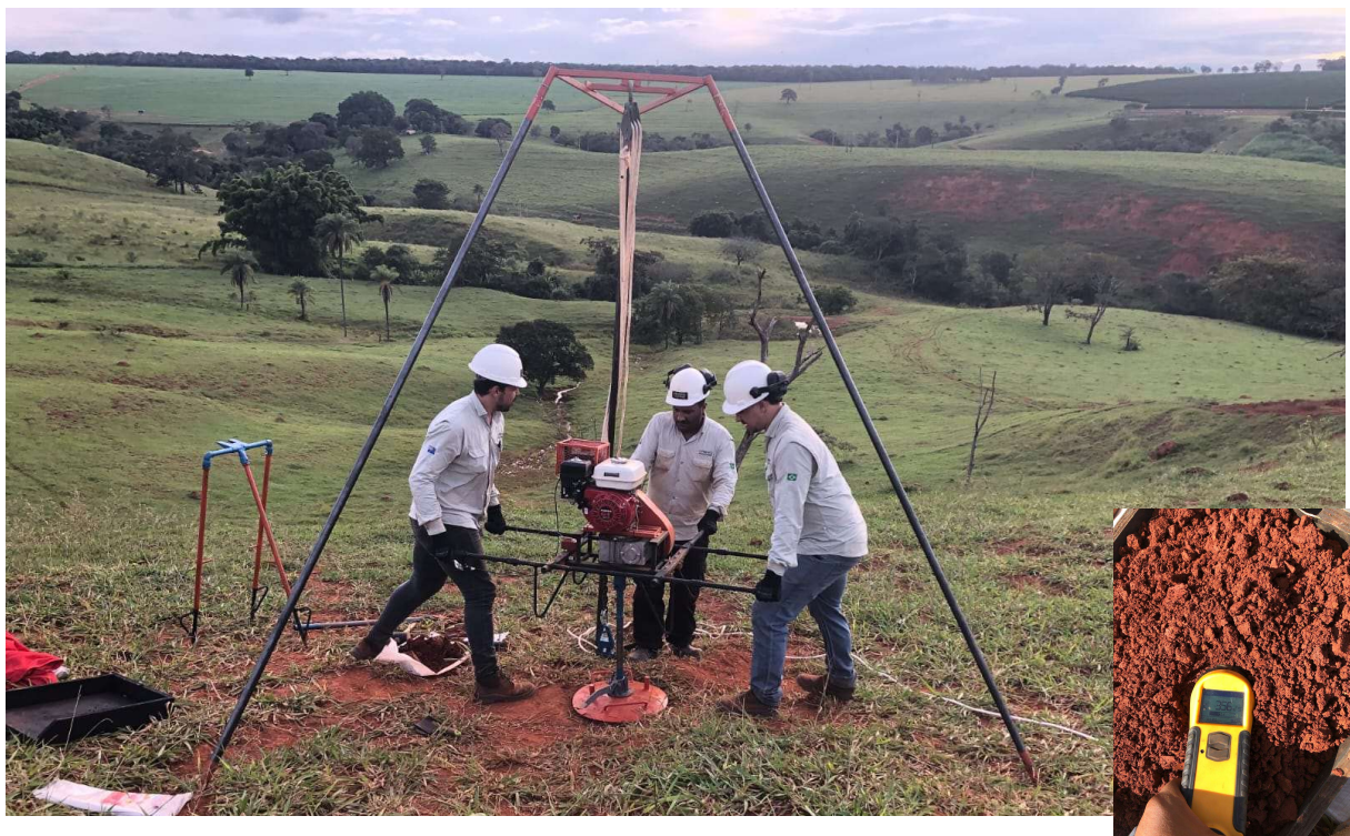
Figure 3: Exploration team drilling at CODA Central (main) and checking magnetic susceptibility of cuttings from auger hole CDC-AD-0001 (Inset)
