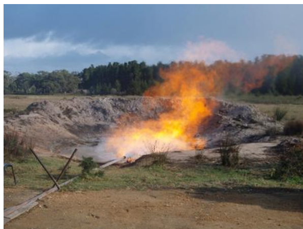
Figures 3 and 4 – Flaring of the gas from the Wombat-2 well
