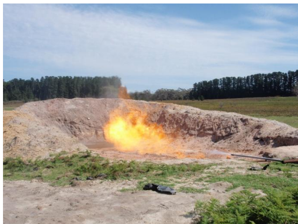
Figures 3 and 4 – Flaring of the gas from the Wombat-2 well
