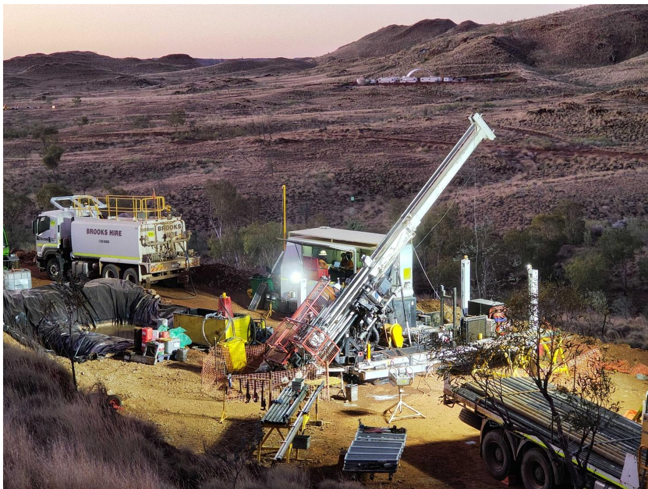
Photo 2. DDH1 Rig #83 capable of low-angle drilling setup on hole 25MYDD028 drilling BIF-hosted mineralisation at Main Hill.
