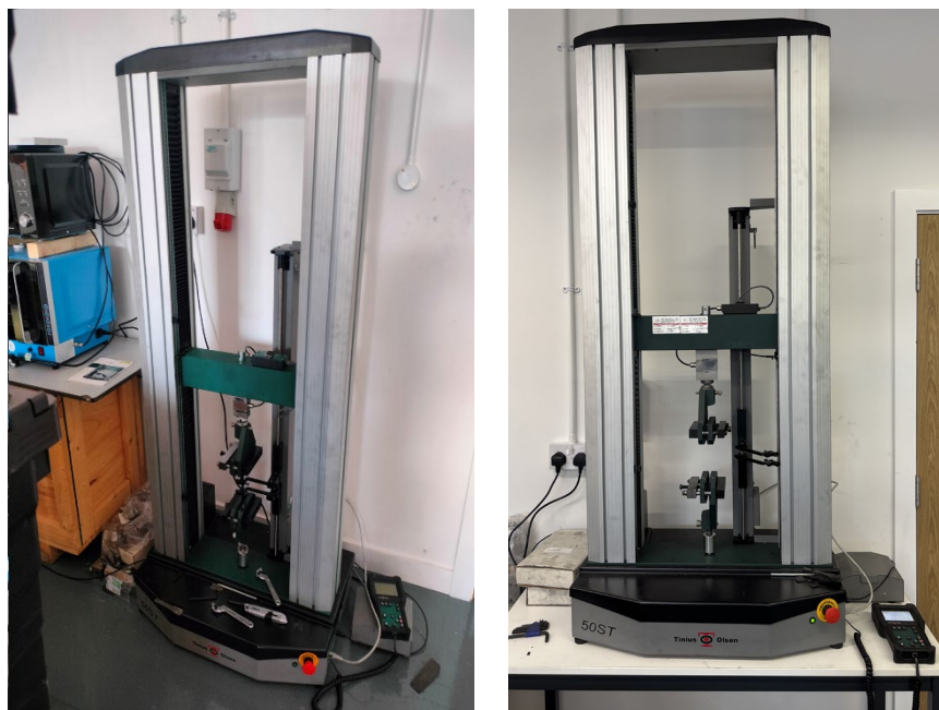
Figure 2: The Tinius Olsen Universal Tester is designed to test graphene-enhanced resin systems for use in storage tanks.
