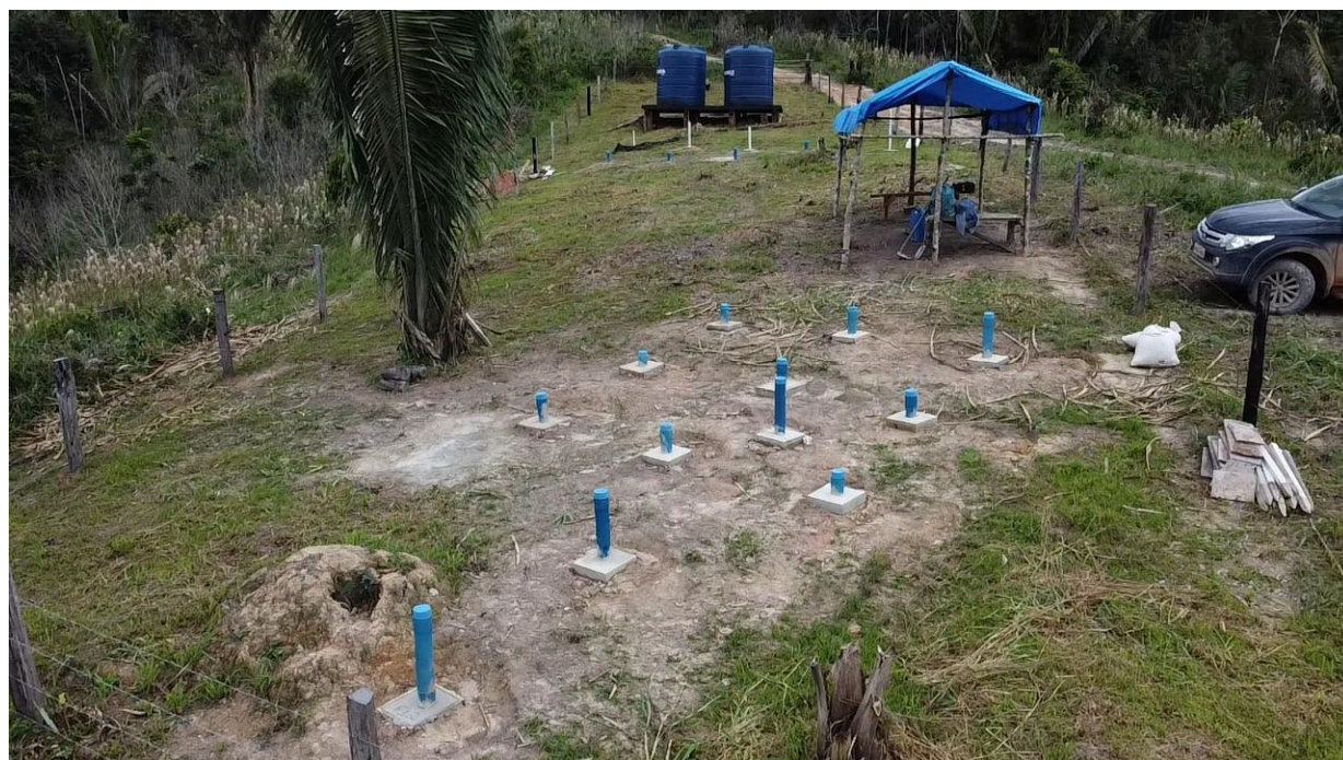
Figure 4. View of the field trial injection and extraction wells, water storage and solution preparation tanks and distribution system where solutions samples were sourced.
