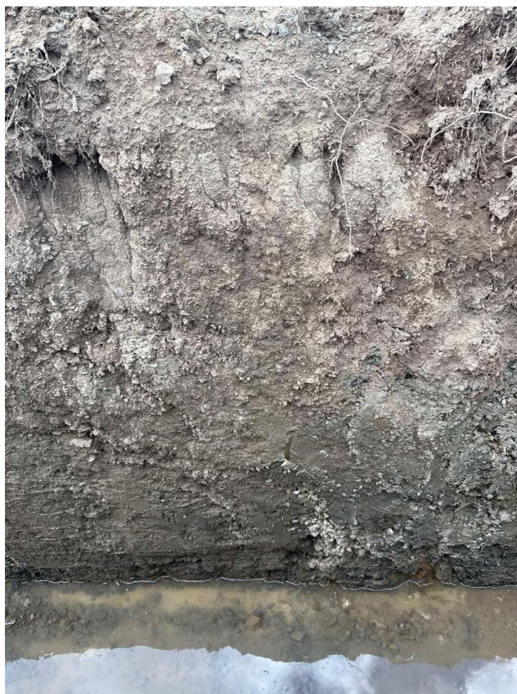
Figure 3 – 2m high trench wall showing completely weathered diorite at 38-39m where copper grades peak at 0.20% Cu.
