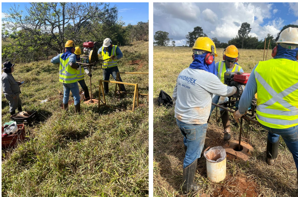
Figure 4 – Auger drilling underway at the Araxa Project.
