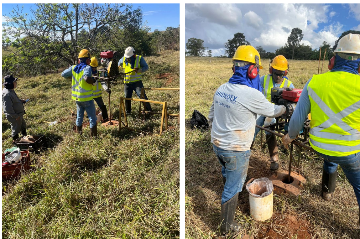
Figure 4 – Auger drilling underway at the Araxa Project.
