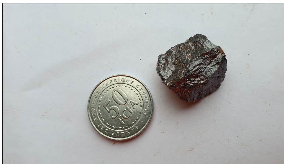
Figure 11: Rutile nugget (22mm) collected up-stream (UTM_84_32N 739273 408418) from stream sediment sample GRMST0001. The visual representation of heavy mineral (HM) and rutile mineralisation shown in this release is based on preliminary visual reconnaissance with no sampling results. Assay results are pending and have not yet been verified through laboratory analysis. Investors are cautioned that the information is indicative only and should not be relied upon as a definitive measure of mineralisation or economic potential. Further exploration and analytical testing are required to confirm the extent, grade, and economic viability of the mineralisation.
