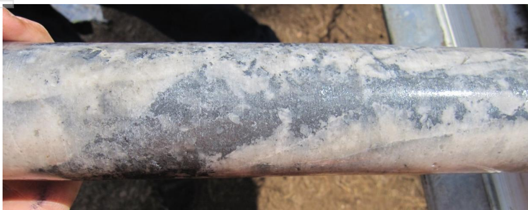
Figure 2. Stibnite-Quartz mineralisation in diamond drill core, from hole CNDD001.
