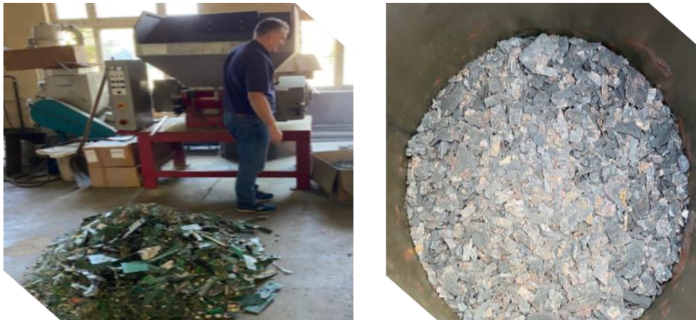
Figure 2: Photo of (L) original E-Waste PCB waste & (R) metal rich char (E-Waste with plastics removed by separate process)
