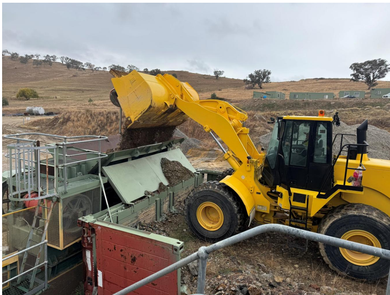
Figure 1: Loader tipping remnant high grade ore to crushing circuit.
