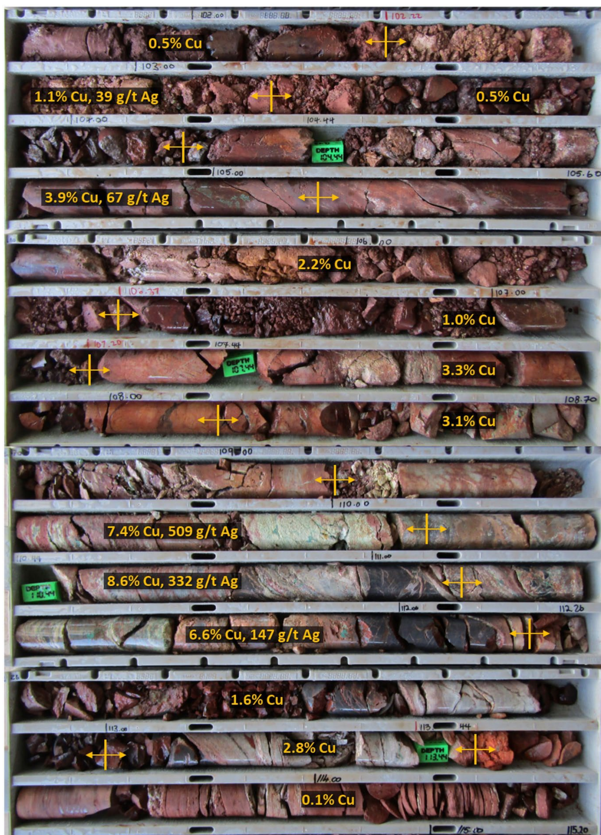
Photo 2: 'NAOTVDD00112' (108.7m - 114.3m), Oxide-Transition Mineralisation
