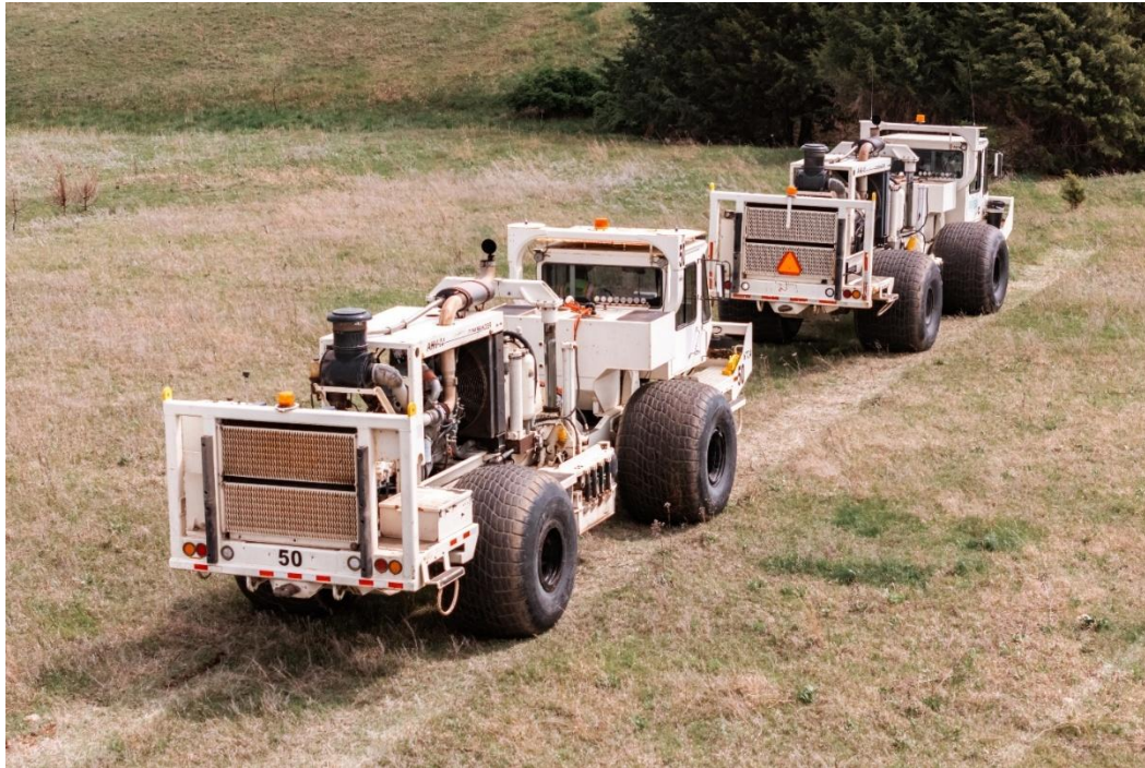
Figure 3: Paragon Geophysical Vibroseis trucks on location within survey area.
