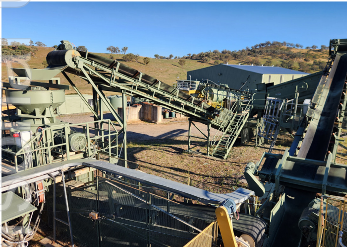
Figure 1: The crushing and milling circuit has been repaired, tested, restarted and repainted. It is now operational.
