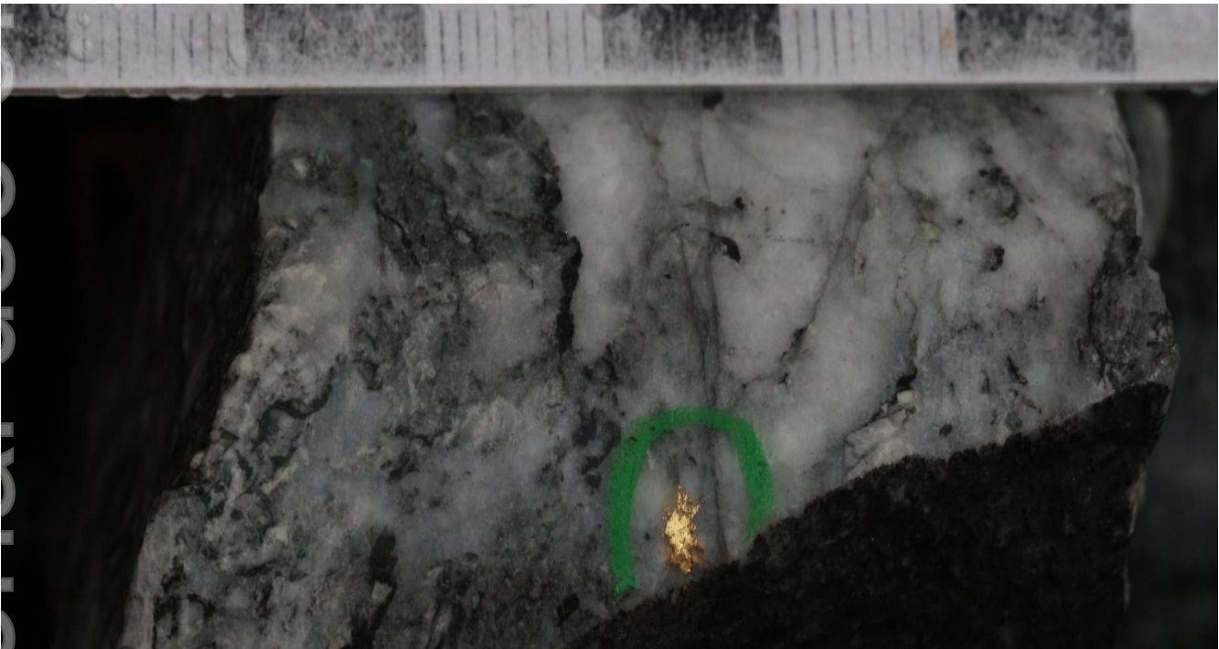
Figure 1 NDS057 – approx. 108.20m – gold (circled). A multiple-phase hydrothermal siliceous breccia includes multiple blebs of visible gold. scale bar in cm's. See also ASX:NSM 19 Mar 25 .
