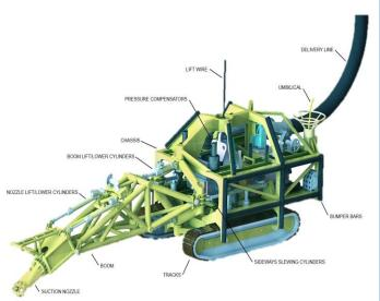
A mobile seabed crawler has been selected as the preferred sediment extraction technology to be integrated into the IMV
