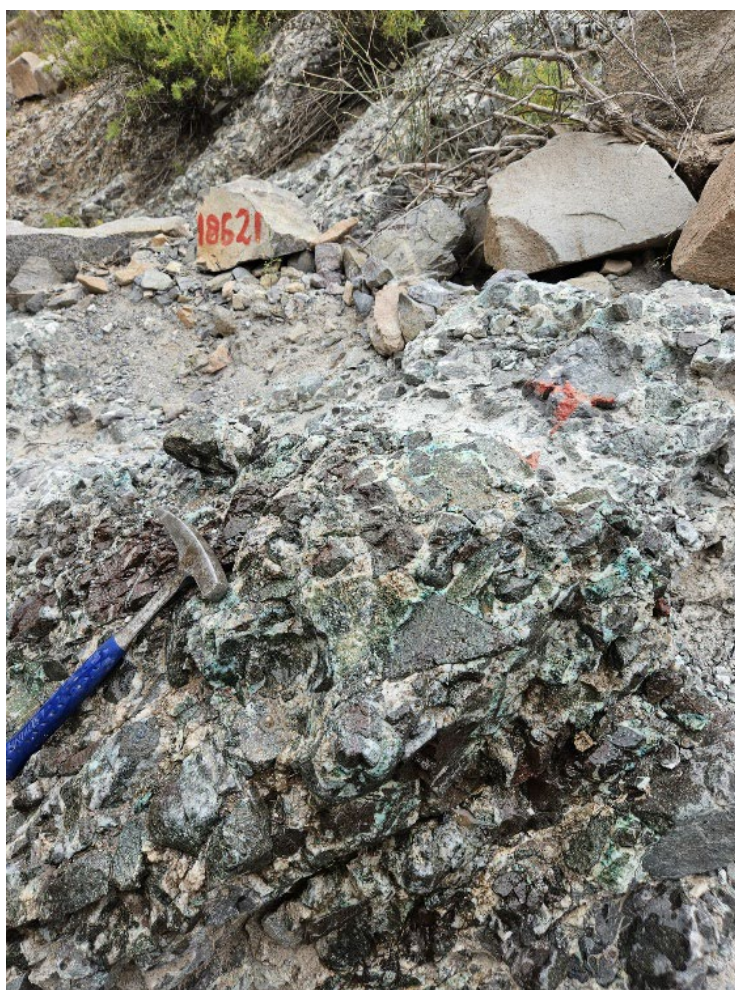
Figure 4: Intrusive hydrothermal breccia with angular, poorly sorted volcanic clasts and a quartz breccia matrix with Cu oxides. Channel 11. Sample 18621 – 335710E, 8079715N. Assays 0,011g/t Au, 1.4g/t Ag, 0.22% Cu.
