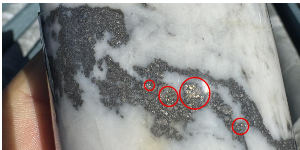
Figure 1. Diamond drill core from AMD003 at 180.0 metres down hole showing abundant grains of visible gold (yellow) hosted within an arsenopyrite vein (grey) in milky quartz. This interval graded 0.7 metres at 446g/t gold from 179.6m.
