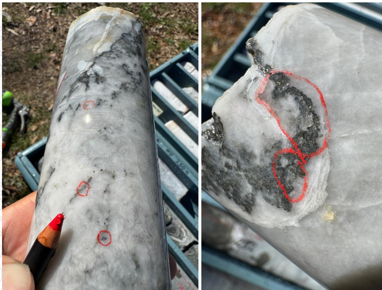
Figure 4. Composite image of core from AMD004 showing visible gold 3 hosted with minor sulphides in quartz. Assay results for AMD004 are currently pending.
