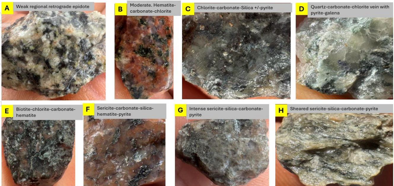
Figure 5 Selection of RC drill chips highlighting the various types of alteration in the granodiorite host rock.
