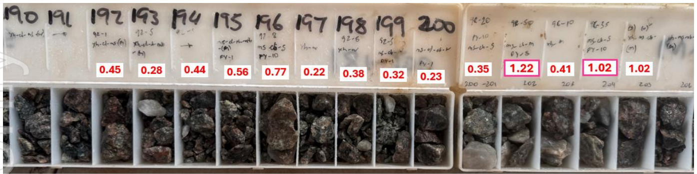
Figure 3 GUYRC0005 (189m to 206m) displaying large, broad, pervasive hematite alteration (189m to 200m) and sericite silica altered zone (200 to 204m). Large broad zone of mineralisation 15m at 0.47g/t within the granodiorite host rock. Numbers in red (g/t) superimposed on the chip trays are the reported gold assays grades over each representative sample interval.
