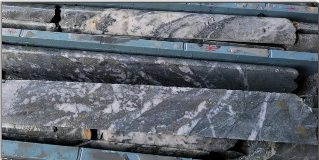
Figure 1. Haunted Stream drilling 2 , ERN001 from 39m with laminated quartz-sulphide vein and brecciated sulphidic sandstone. The hole intersected 13m @ 3.57 g/t Au from 39m.
