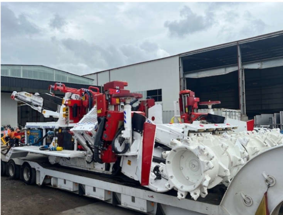
Continuous Miner post overhaul and ready for delivery to Malabar, Kurri Kurri (NSW) facility.
