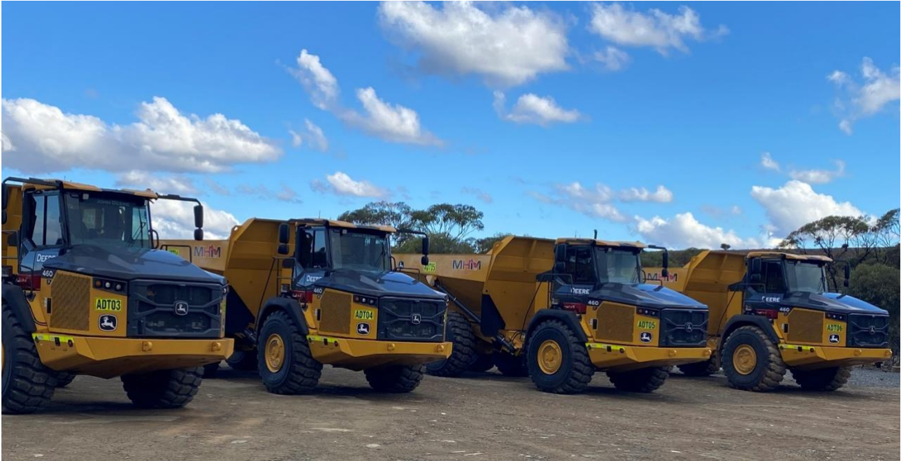
Photo 1: MHM Contracting 40-tonne Moxy dump trucks on site at Munda Gold Mine.
