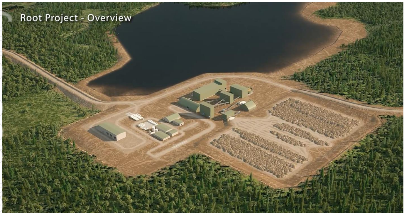
Figure 1: Rendered Root Project layout model showing views of processing plant, mining, and water management infrastructure
