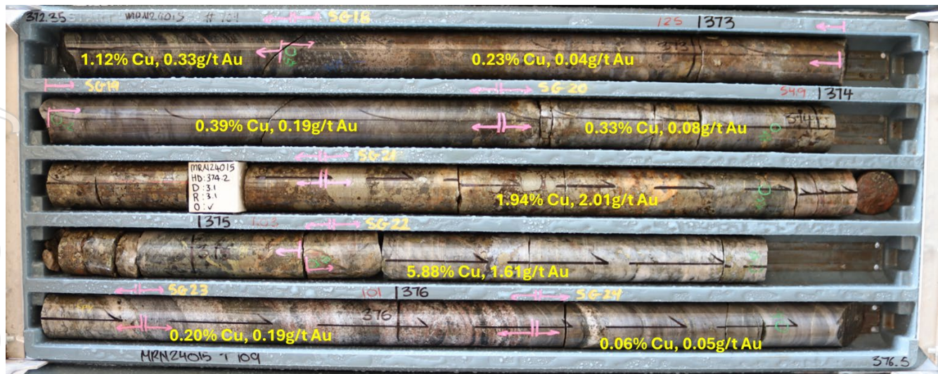
Figure 1. Photo of high-grade copper intercept in MRN24015 – 1.47m at 3.55% Copper, 1.85 g/t gold, 16 g/t silver from 374.25 metres
