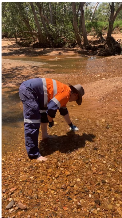
Figure 2. Baseline surface water samples being collected from the Fullarton River
