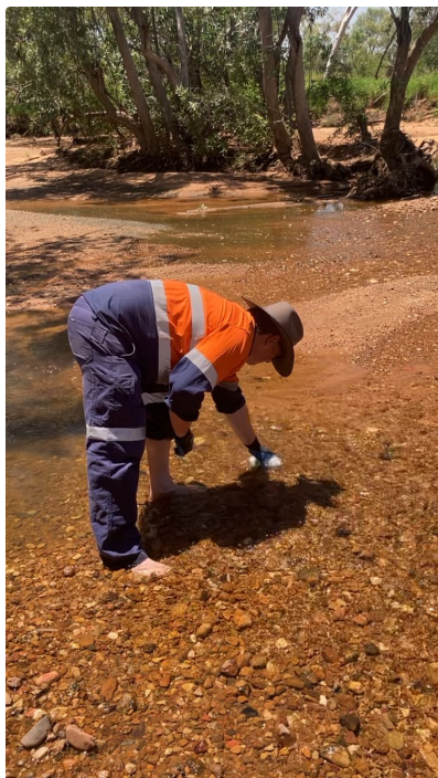
Figure 2. Baseline surface water samples being collected from the Fullarton River
