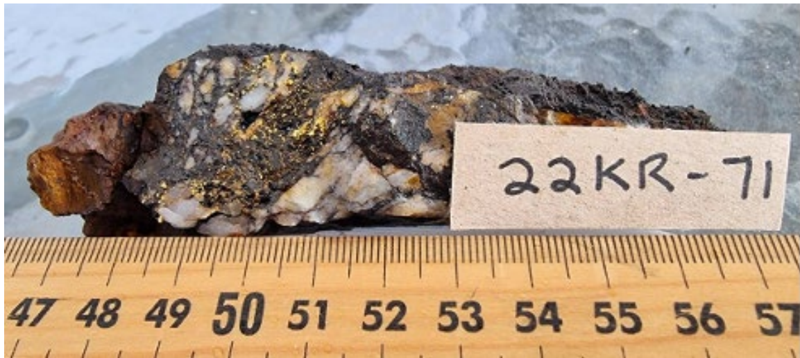
Figure 4: Birdsnest Prospect costean sample 22KR-71 grading 44,072 g/t Au & >5,000 g/t Ag (ASX Announcement: 15 December 2022) 1 .
