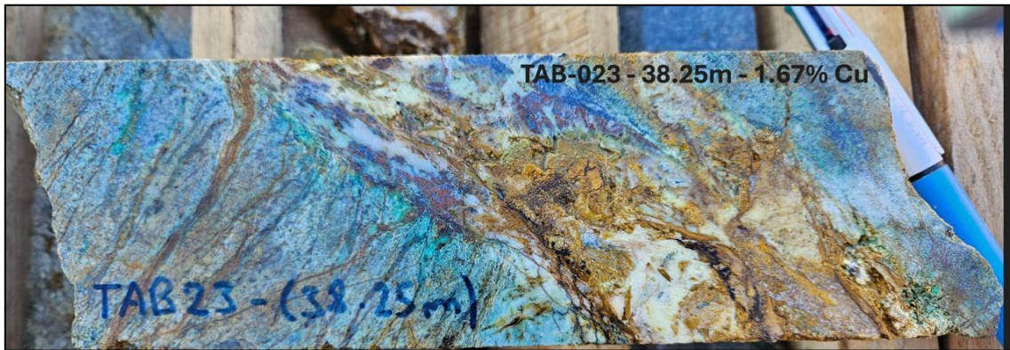
Image 2: TAB 023 – Brecciated metasediment containing Cu oxides (atacamite, chrysocolla and disseminated copper wad along fractures and clast rims) 3
