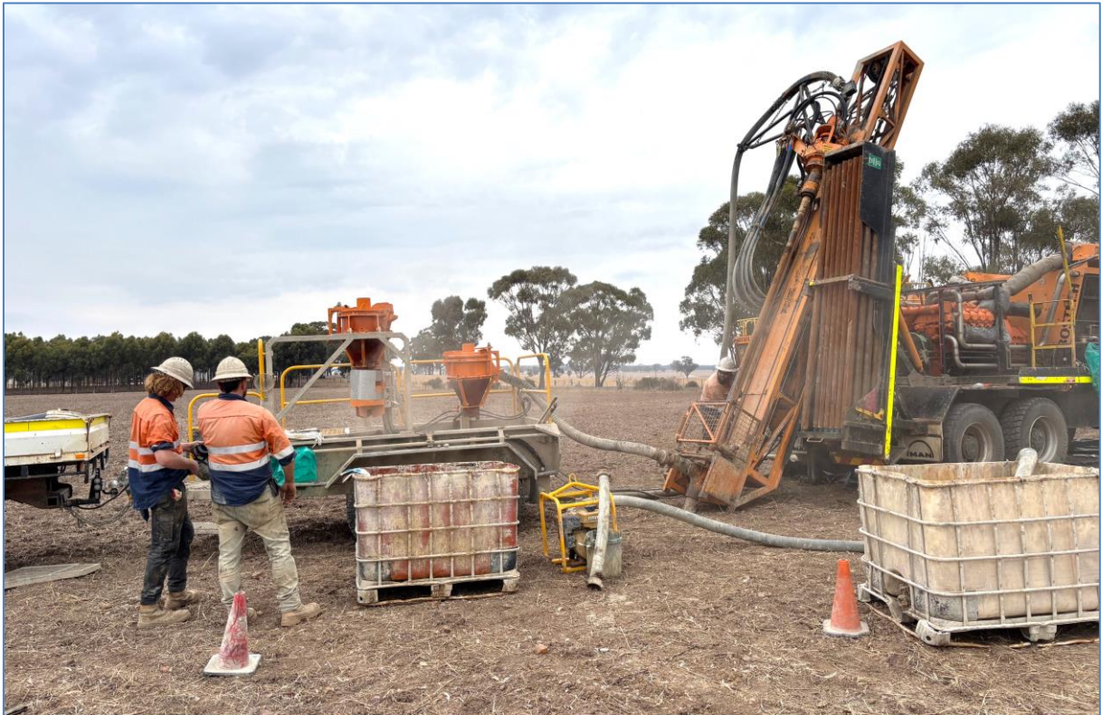
Figure 3. Photo of aircore drilling operations at Fosterville.
