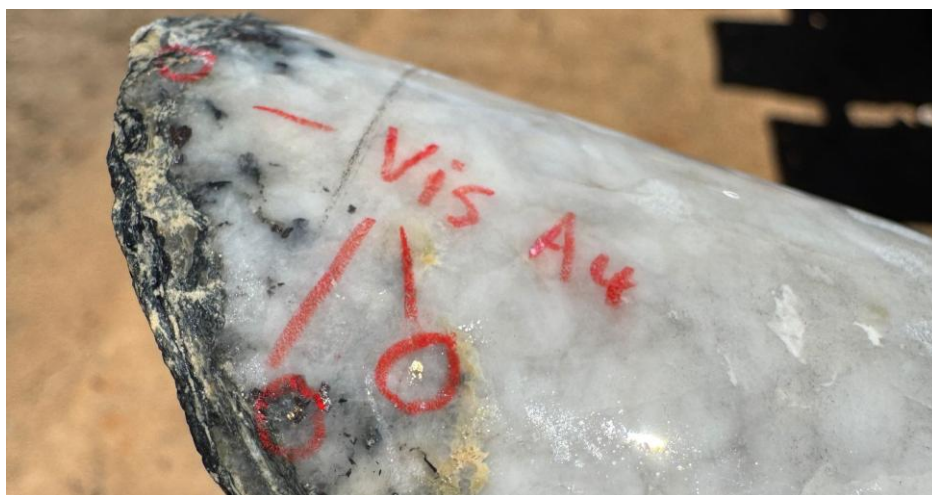
Figure 8. Visible gold mineralisation (assays pending) in patches to 3mm with minor sulphides hosted in quartz from recent drill hole AMD001 at 158.7m downhole (ASX AVM 25 February 2025).
