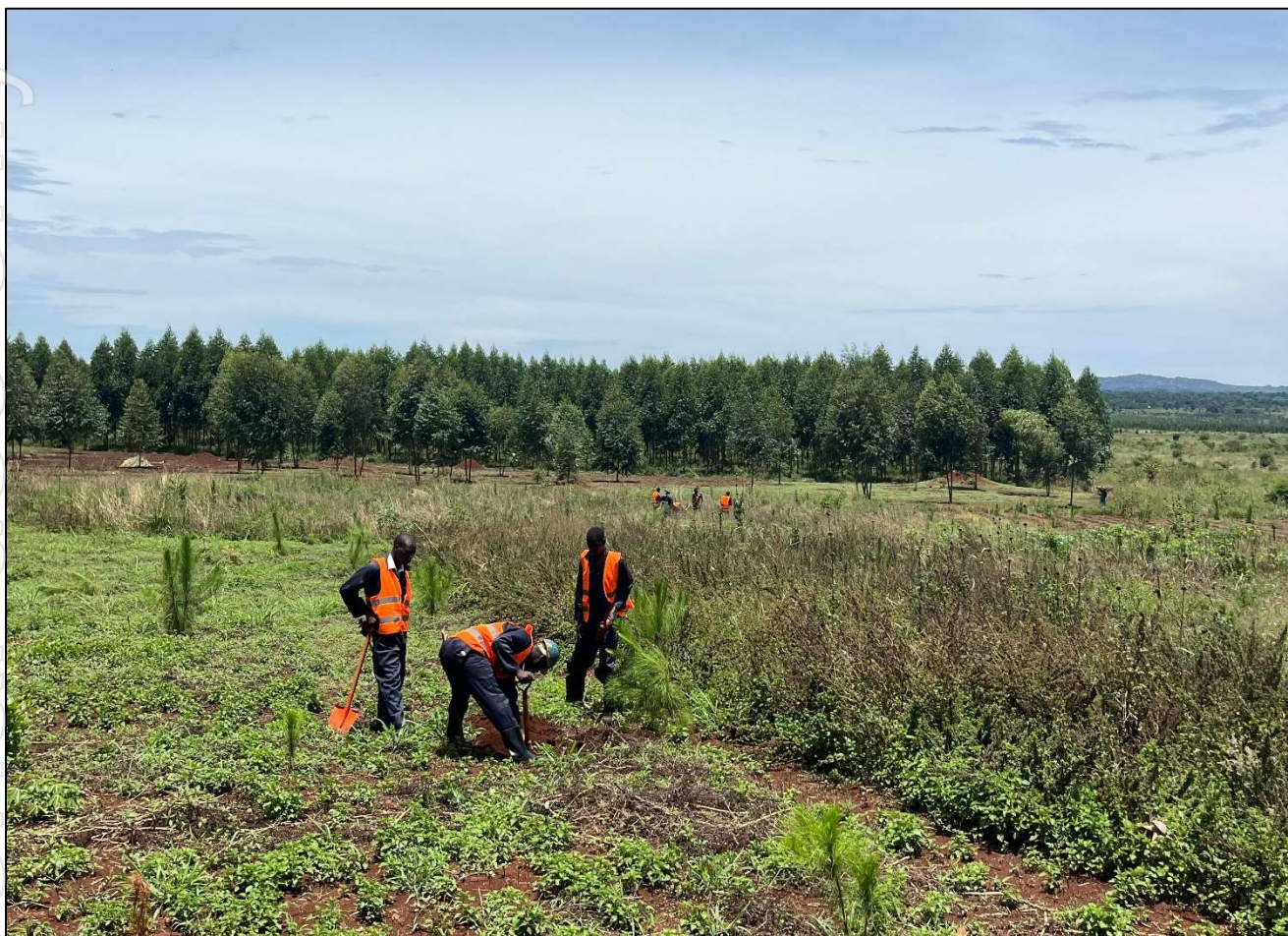
Figure 2: Field crew digging a hole to the B-horizon to take a soil sample.
