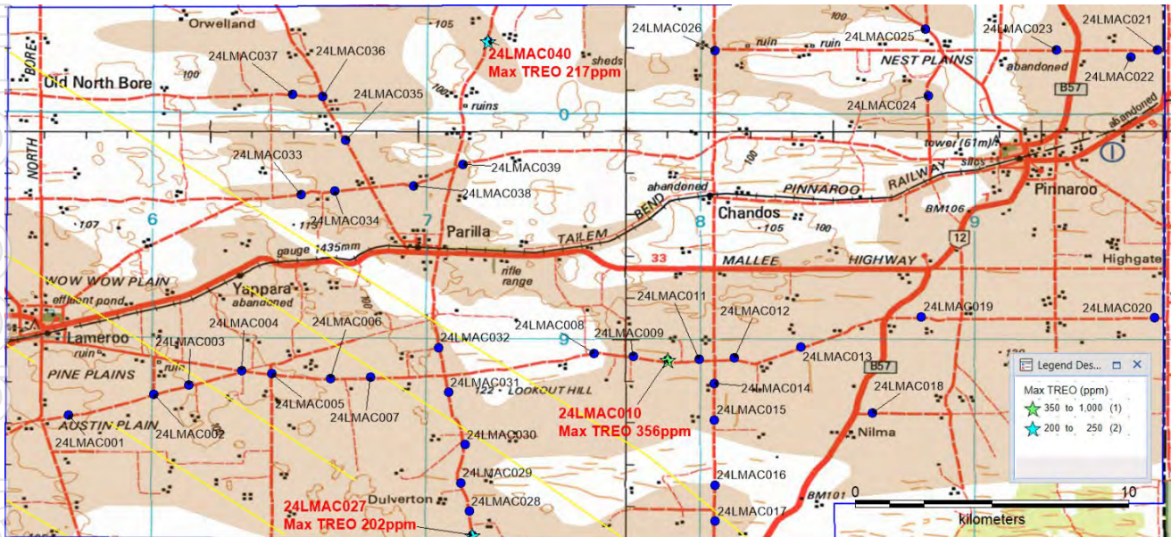
Figure 3: Location of Lameroo Aircore Drill Holes (LM series) within the target Loxton/Parilla Sands (brown) and showing maximum ppm TREO in the hole
