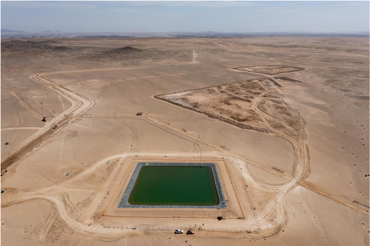
Figure 3: Water storage facilities on site will provide 10 days' storage capacity, significantly minimising the risk of any potential disruptions.
