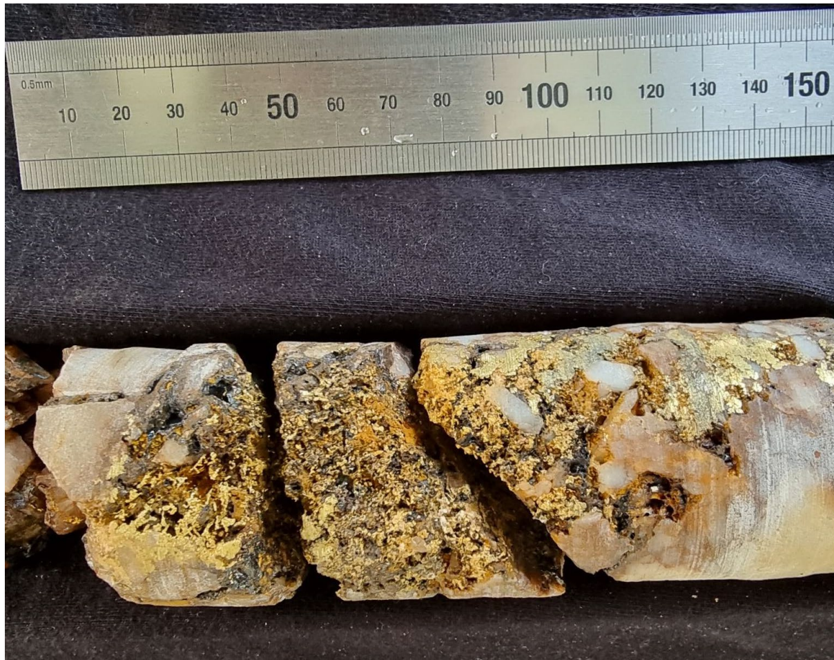
Figure 3: Peninsula Prospect - At surface drill core photo of 'Hole A' (ASX Announcement 5 August 2022). To assist with mineralogical and textural studies at the Newman Project, Hole A was not split and assayed for gold (ASX Announcement 12 January 2023) 1 .
