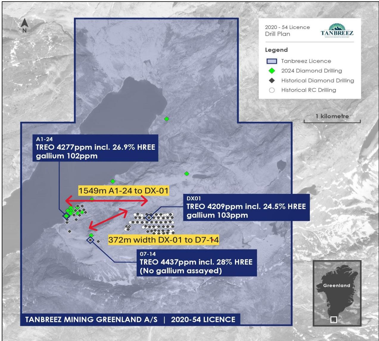
Figure 1 Drillhole collar positions for deep diamond holes DX-O1 to 338m, D7-14 to 243m and A1-24 to 40m with the average assays results from surface. The length between drill holes is 1549 metres from A1-24 to DX-01 and 1037m from DX-01 to D7-14 with a 372m width between DX-01 and D7-14.
